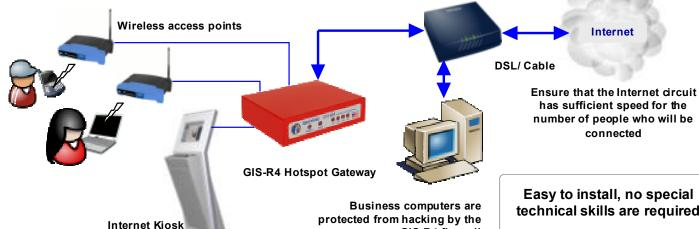
Use Guest Internet gateways with any type of wireless access point. Wireless access points are installed throughout the premises to ensure good wireless coverage
