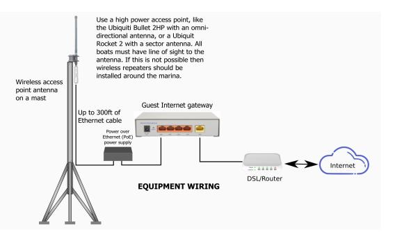
The Guest Internet gateway is installed in the main office together with the DSL or Cable router. An Ethernet cable runs from the gateway LAN port to the power injector for the wireless access point, and then along another Ethernet cable up to 300 feet in length. This cable runs up a tall mast with the wireless access point installed at the top of the mast. The wireless access point should be above the height of adjacent trees to ensure good signal transmission.
